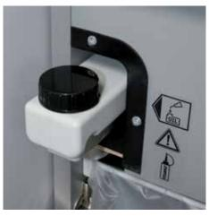
Integrated oil tank for controlled, automatic lubrication of the cross-cut cutters helps to lengthen service life while keeping performance constant
